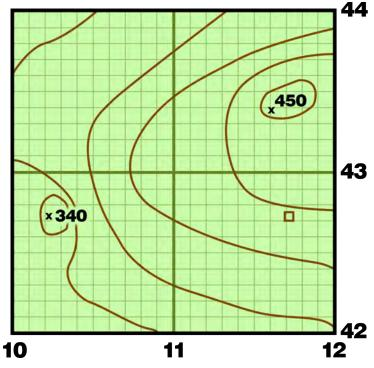
Determining a Six-Digit Grid Coordinate
