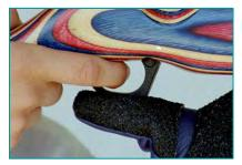
Take up the slack (first-stage) on the trigger and then, with the sights aligned on the target, smoothly press the trigger to the rear until the mechanism releases.
