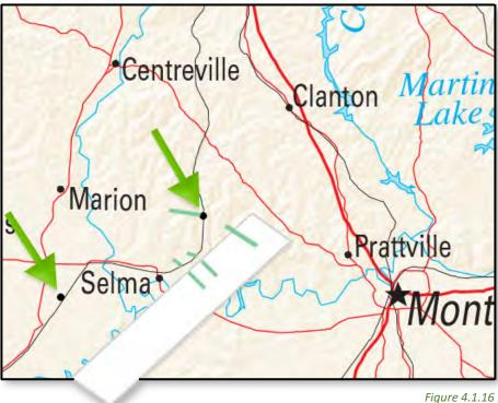
Keep pivoting and marking points until you reach your destination on the map. To find the distance, line up your marked straightedge paper with the map bar scale. Now you can measure the distance between your first and last marks to find the distance of the curved route.
