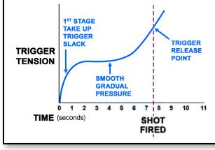
This graph shows how pressure is applied to the trigger. The time from the first application of pressure until the mechanism, releases should last about 4-8 seconds.
