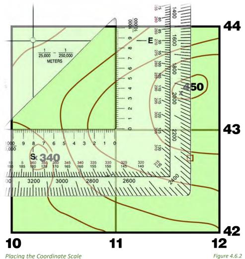
3. Keeping the horizontal scale on top of the <u>43</u> grid line, slide the scale to the right into the grid square until the vertical scale intersects the center of mass of the spot elevation. (See Figure 4.6.3)
