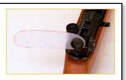
A rear sight blinder can be made from a piece of translucent plastic. Cut a hole in one end so that the blinder will fit over the detached rear sight iris.
