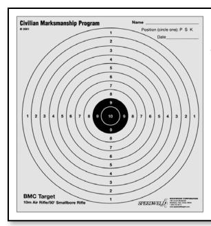
The BMC target is printed on a 6 1/2"x7" card, has a 15.25mm 10-ring and nine additional scoring rings that are each 15.25mm larger.
