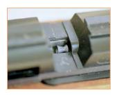
Complete loading by pushing the bolt forward to the seat pellet in breech.
