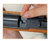
To load the Daisy M853/M888, place a pellet in the loading port and close the bolt by pushing it forward.
